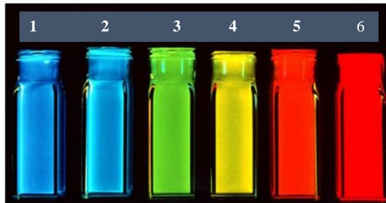
Figure 3: CdSe QDs irradiated with a UV lamp. From left to right, samples were taken as the synthesis progressed.
